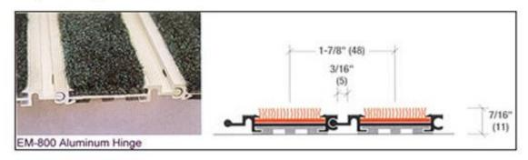
CONSTRUCTION: A series of aluminum tread rails spaced at 1 7/8", O.C. connected by a black vinyl hinge or mill finish aluminum hinge; supplied with a square aluminum edge, a black square vinyl edge or a black beveled vinyl edge around the perimeter. Both style hinges are available solid or perforated.
