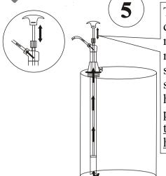
Take an empty container & place it below the discharge spout. Start operating the pump handle by moving it up by about 12" & then down. Within a maximum of 4 strokes, pump will be primed & will start dispensing media. Amount of fluid discharge per stroke can be controlled by the lift of the pump handle. The higher the lift, the greater the discharge per stroke. Never take the pump handle to its extreme top position, but operate within a convenient lift height.
