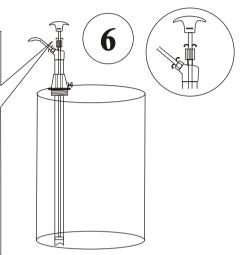
Due to the nature of aggressive media with which this pump maybe used, it is designed to drain out all the fluid from the pump body, when not in use. Pump needs to be re-primed each time it is used & this generally takes only 2-3 strokes
